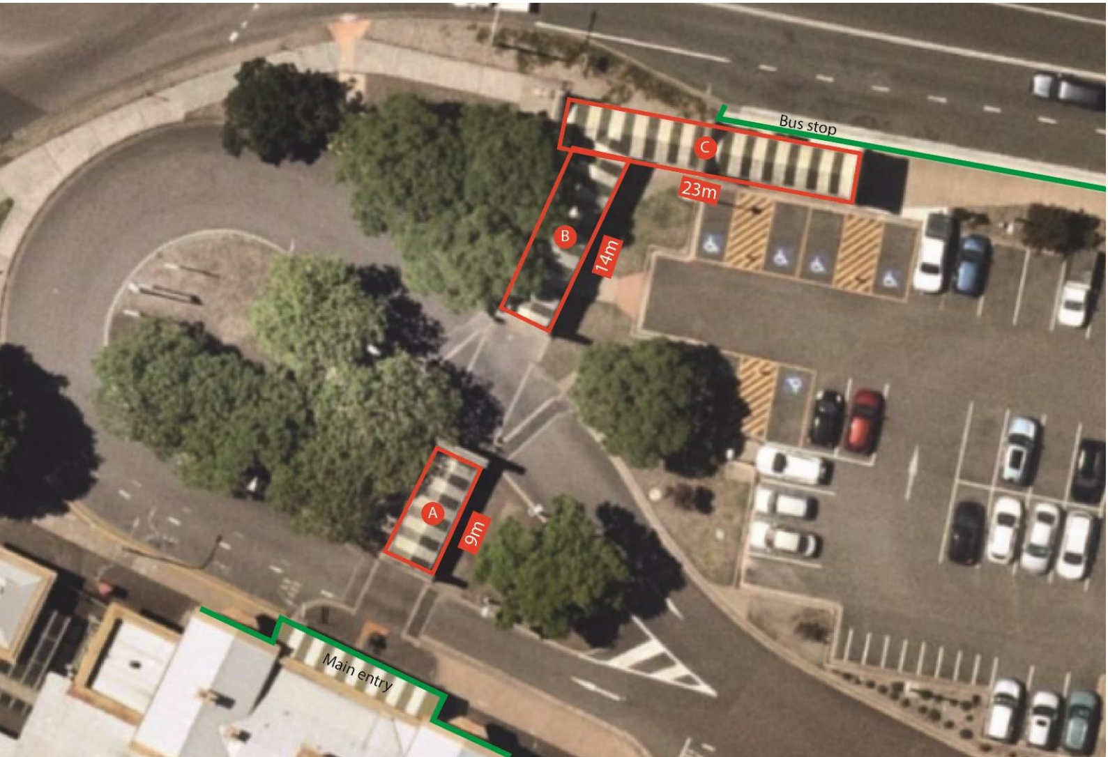
Aerial image showing covered pedestrian walkway, inclusive of measurements
